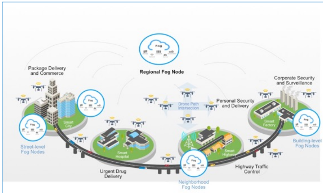
Figure 8: illustrates a fog computing infrastructure for supply chain delivery in a smart city. The hierarchy helps ensure dynamic flight plans, air traffic control database updates, and up-to-the-second weather reports while the aerial drones are in transit.
